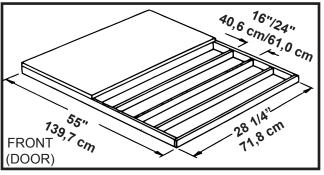
Note: Platform/Slab will extend 9/16" (1,4 cm) beyond floor frame on all four sides. Seal this 9/16" (1,4 cm) of wood with a roofing cement (not included), or bevel this 9/16" (1,4 cm) of concrete when pouring, for good water drainage.
