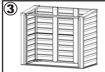
Install Side Channel, Rear Channel, & Lintel
