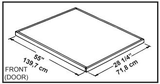
Note: Finished Slab dimensions, with lumber removed.
