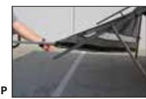
**Step 4:** Reduce each leg to its lowest position by unlocking the latch and then retracting the leg. Once retracted, lock the latch to hold the leg into place (Fig. Q).
