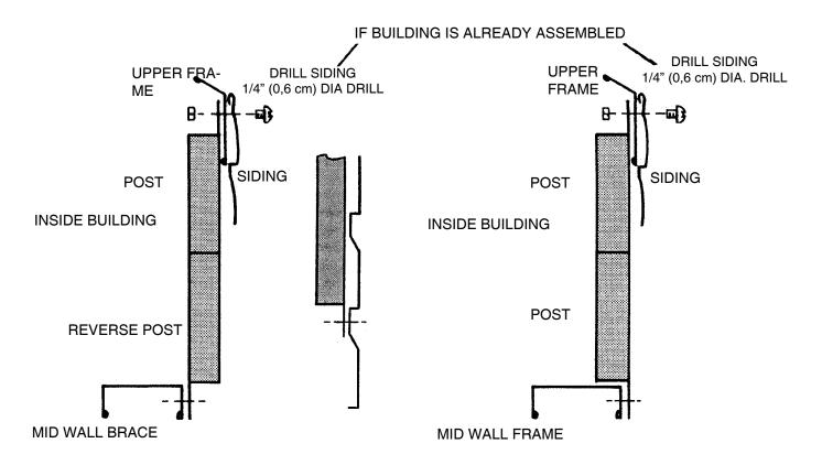
FOR BUILDINGS WITH NO MID WALL FRAME: Telescope posts to line up tab on bottom post with flat spot in siding panel. Fasten posts together with a bolt and nut. Using hole in bottom tab as a guide, drill 1/4" diameter hole through siding panel and fasten using a bolt and nut.
