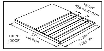
Note: Platform/Slab will extend 9/16" (1,4 cm) beyond floor frame on all four sides. Seal this 9/16" (1,4 cm) of wood with a roofing cement (not included), or bevel this 9/16" (1,4 cm) of concrete when pouring, for good water drainage.
