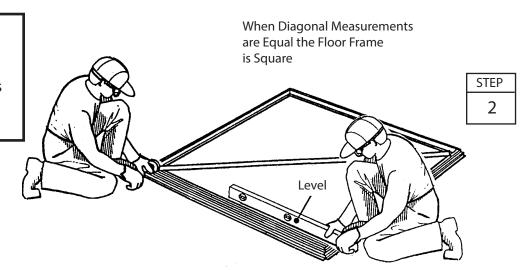
The floor frame must be square and level or holes will not align.
