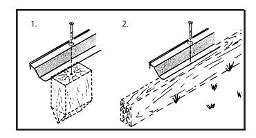
**Arrow Anchoring Kit:** (Model No. AK100 or 68383) Recommended for use with the concrete base. Contains: Corner gussets, perimeter clips, hardware, 1/4" masonary drill bit and installation instruction.
