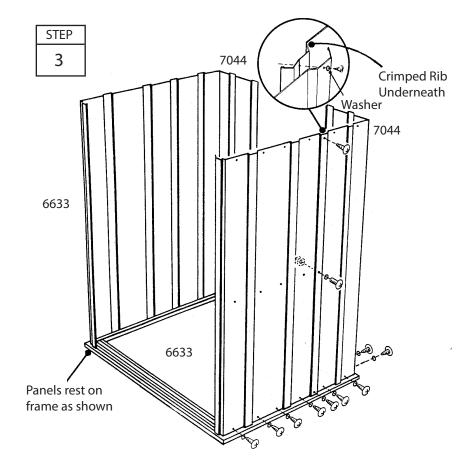
The main frame pieces give rigidity to the side and rear walls and provide a surface for attaching the gables which support the roof.
