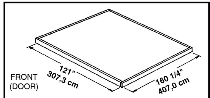
**Allow 3 - 5 hours for construction and a week for concrete curing time.** Note: Finished Slab dimensions, with lumber removed.
