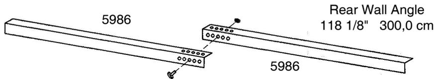
**3** Overlap the **rear wall angle** pieces as shown in the figure and fasten them together with *one bolt in the center hole*.
