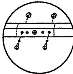
Use bolts and nuts thru wall angle overlap at the top of panel at rear.
