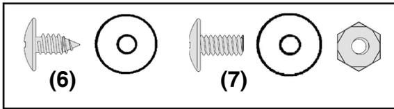
Installing the roof panels is best done with a step ladder. Install the first roof panel at the back right corner of the building. Each screw and bolt in the roof requires a washer.
