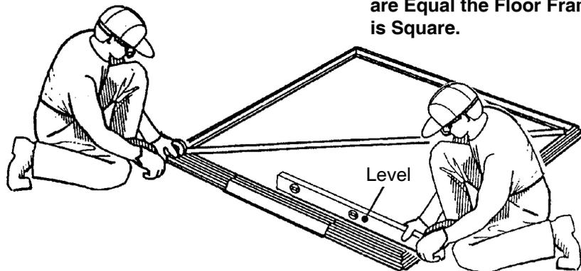
**The floor frame *must be square and level* or holes will not align.**
