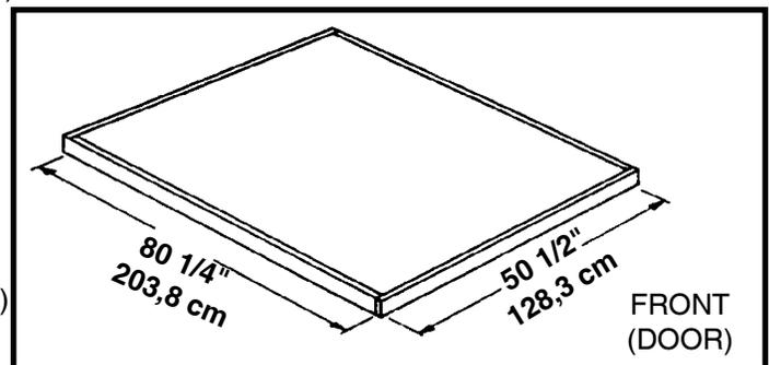
**Note:** Finished Slab dimensions, with lumber removed.
